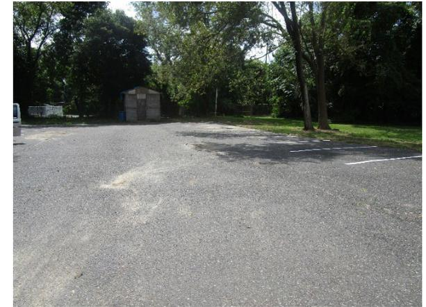
The section of parking spaces on the south side of the property can be replaced with pervious pavement to capture and infiltrate stormwater runoff from the parking lot. A preliminary soil assessment suggests that the soils have suitable drainage characteristics for green infrastructure.
